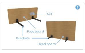
2. Assemble the board holders 3 & 4 to the new headboard 1 and footboard 2 for full length rails. Ensure the brackets are orientated towards each other as shown and are mounted to the same side of the board as the aluminium tracks.
