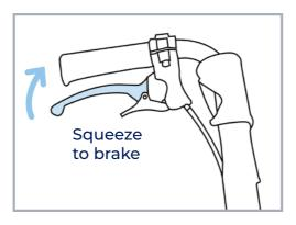
**BRAKE:** To engage brakes, squeeze the handbrake in an upwards direction.
