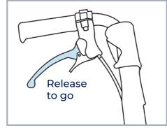
**RELEASE BRAKE:** To disengage brakes, release the handbrake.
