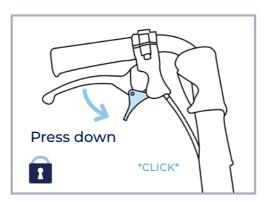
LOCK: To engage brakes, squeeze the handbrake in an upwards direction. Press down on the switch until it clicks, this will lock the brakes.
