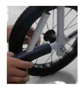
The anti-tip wheel height range is adjustable for improved mobility during carer transportation.
