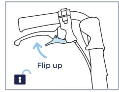
**UNLOCK:** To disengage brakes, flip the switch upwards.
