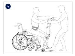
Once the user is standing upright with their center of balance close to the handle, attach the standing sling to the sling retaining hooks on the handle. Bring the outer straps of the sling around the handle (above belt retaining pegs) and secure by clicking the safety buckle into place.
