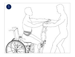
4. Ask the user to position their feet on the footplate, then grasp the Grab bar and stand up with lower legs against the Knee Pad for support. The caregiver can provide minimal assistance by using the handles on the sling to guide the person into standing.
